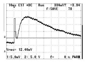
**Fig. 4.** An example of the oscilloscope display in the present study. Channels 1 and 2 were used to monitor thermocouple output and voltage for impulse heater (see Fig. 1b), respectively. Note that the Channel 1 data were magnified 1000 times by a DC amplifier. The corresponding digitized data of Channel 1 were used for curve fitting to determine parameters *A* and *B* in Eq. (2).
