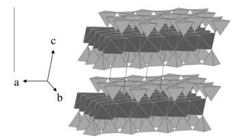
**Fig. 1.** Crystal structure of talc. It is composed of layers of tetrahedron and octahedron sheets. Si and Mg atoms are inside the tetrahedrons and octahedrons, respectively.
