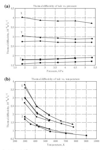
**Fig. 5.** Thermal diffusivity results. (a) Pressure dependence. (b) Temperature dependence at 5.3 GPa. The temperature dependence was measured during temperature decreasing process in multiple heating. Triangle ( $\blacktriangle$ ), circle ( $\bigcirc$ ), and square ( $\blacksquare$ ) symbols correspond to *X*, *Y*, and *Z* directions, respectively, of the present talc block.
