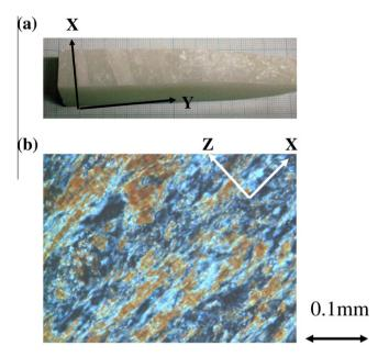
**Fig. 2.** (a) Photograph of a block used in the present work. The *X* and *Y* directions are specified by arrows. The *Z* direction is normal to the foliation surface. (b) Polarized microscope view on a thin section in the *Y* direction. *X* and *Z* directions are specified by white arrows. Note the relatively fine grain texture.
