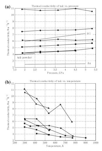
**Fig. 6.** Thermal conductivity results. (a) Pressure dependence. The dotted line is the data for sintered talc from powder (Gummow and Sigalas, 1988). The dashed lines are olivine (OI; Osako et al., 2004) and antigorite (An; Osako et al., 2010) data, as references. (b) Temperature dependence at 5.3 GPa. Triangle ( $\blacktriangle$ ), circle( $\bigcirc$ ), and square ( $\blacksquare$ ) symbols correspond to *X*, *Y*, and *Z* directions, respectively, of the present talc block.
