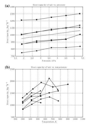
**Fig. 7.** Heat capacity results. (a) Pressure dependence. The dashed line is the average of the six measurements. (b) Temperature dependence at 5.3 GPa. Triangle ( $\blacktriangle$ ), circle ( $\odot$ ), and square ( $\blacksquare$ ) symbols correspond to *X*, *Y*, and *Z* directions, respectively, of the present talc block.
