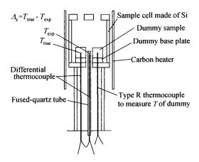
**Fig. 1.** Schematic diagram of the arrangement of the sample and differential thermocouple.
